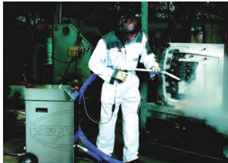
industrial - mould cleaning
